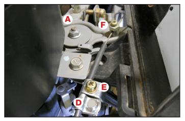
5. Install the new nut and bolt from the kit into the original cable clamp (D). Before tightening the nut pull the cable so the throttle stop screw (F) is butted up against the throttle lever stop tab (A). In this position slide the cable clamp (D) up against the cable clamp (E). Tighten the nut/bolt of clamp (D) securely.
