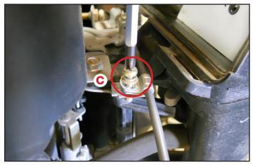
3. Remove the phillips head screw (C) holding the original cable clamp. Save the screw and washer to be used with the new cable clamp (B).
