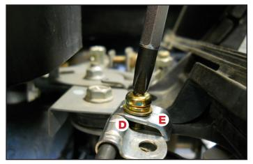
4. Slide the original cable clamp (D) approximately <sup>3</sup>/<sub>4</sub>" down the cable sheating. Secure the new cable clamp (E) with the original phillips head screw and washer. Use blue loctite on threads and only tighten until snug. If assembled correctly the top right corner notch will fit into the notch of the bracket below cable sheating.
