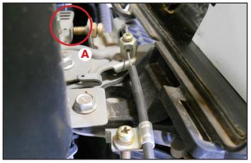
1. Note that the throttle lever stop tab is butted up against the throttle lever stop screw (A).
